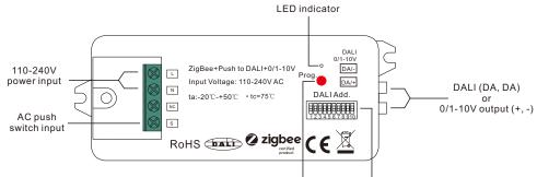
Program key, for network pairing, touchlink and factory reset of the device
