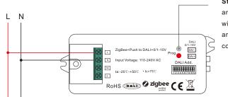
Step 4: LED indicator will blink 5 times and then stay solid on, then the device will appear in your controller's menu and can be controlled through controller or hub interface.
