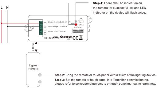
Note: 1) Directly TouchLink (both not added to a ZigBee network), each device can link with 1 remote. 2) TouchLink after both added to a ZigBee network, each device can link with max. 30 remotes. 3) To control through both gateway and remote, add remote and device to gateway network first then TouchLink
