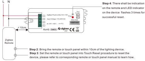
Note: Make sure the device already added to a network, the remote added to the same one or not added to any network.
