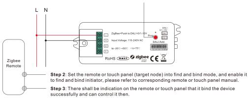
Note: Make sure the device and the remote or touch panel already added to the same Zigbee hub.
