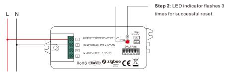
Note: 1) If the device is already at factory default setting, there is no indication when factory reset again .2) All configuration parameters will be reset after the device is reset or removed from the network.
